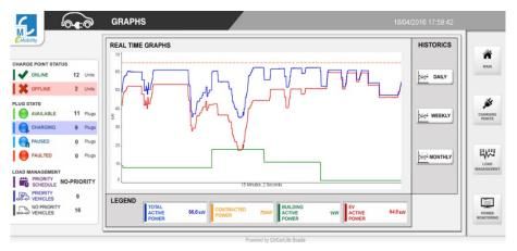
A graph screen should display a graph in real time of the consumption of the building, the EV and the sum of both, compared to the contracted power, giving access to historical graphs.
