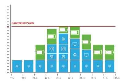
Garage curve example where intelligent system reduces the EV charge to avoid main breaker trip.
