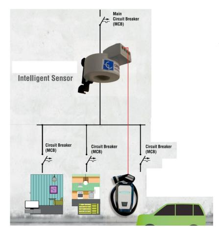
A sensor is to be installed at the main breaker home cabinet to get the real time house power. This sensor will send the signal to the EV charger and it will decide to let the EV get tits full requested charge power or to reduce it until necessary. This is possible only with EV charger type 1 or 2 but not with the existing home garage plug.
