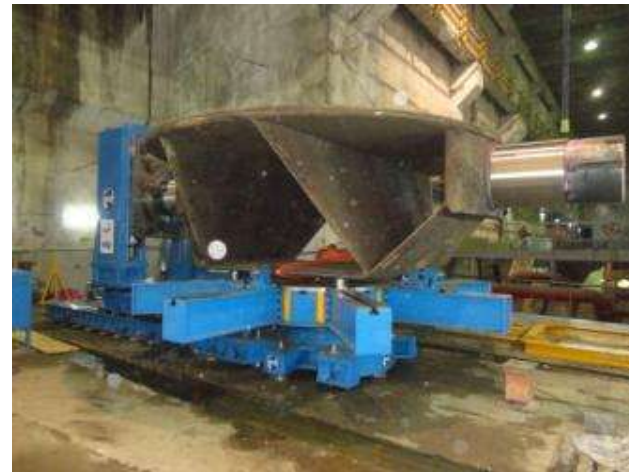
Butterfly valve trunnions machining
