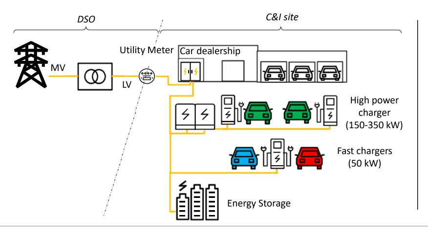
Buffer energy storage enable integration of EV charging infrastructure to the existing grid connection without/with limited impact on PCC
