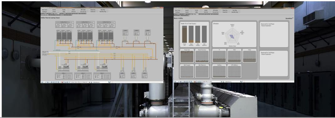
Monitoring and centralised control over facility systems, such as chillers, CRACs, AHUs and the electromechanical plant, including environmental and other physical factors.
