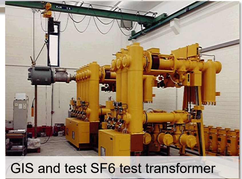
SF6 transformer with coupling capacitor
